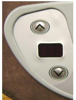
To set the temperature, press the up or down arrow once to display the current setting. Then, use the up (^) and down (v) arrows to adjust the temperature to the setting you desire. The current temperature setting will display for 5 seconds after the up or down buttons are pressed. After this time has elapsed, the display will revert to displaying the water temperature.
